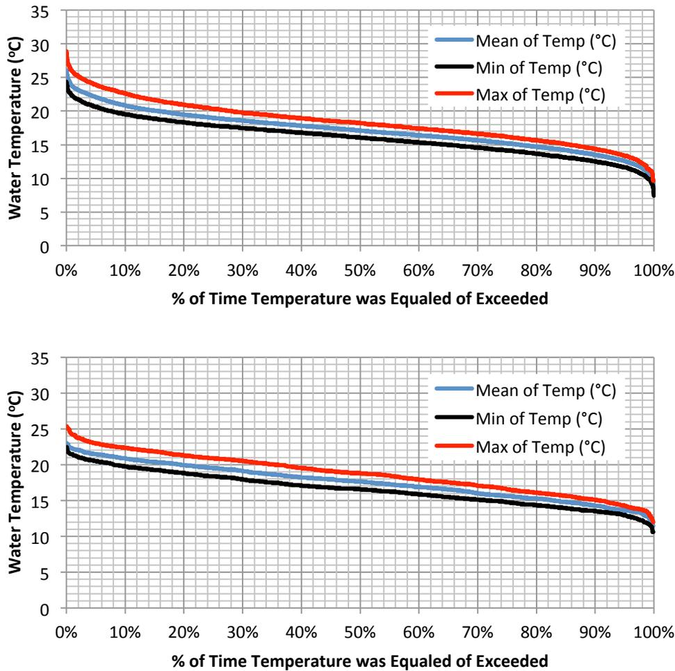
Figure B.1.10. Temperature duration curves for MDFW (upper) and CT DEEP (lower) sites developed from daily stream temperature observations for June, July, and August.
